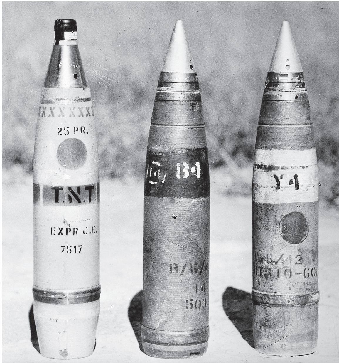
25 pounder shells prior to sea dumping off Sydney. B4 = tear gas, Y4 = mustard gas
