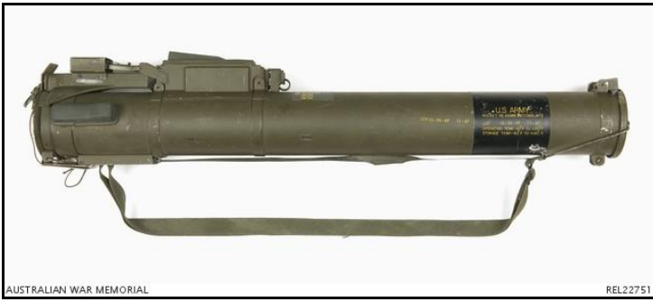
Figure 1 - M72 (L1A2F1) Rocket Launcher in closed/unarmed position (AWM ID REL22751)
