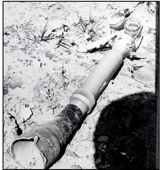
Figure 2 - Fired and ruptured M72 rocket
