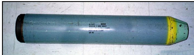
Figure 4 - 5 inch WP rocket warhead (without fuze fitted)
