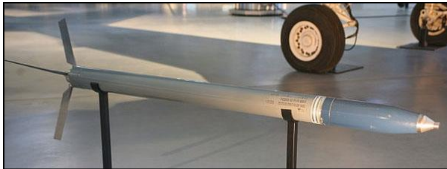
Figure 3 - Complete Zuni 5 inch FFAR (5" rocket and 5" warhead)
