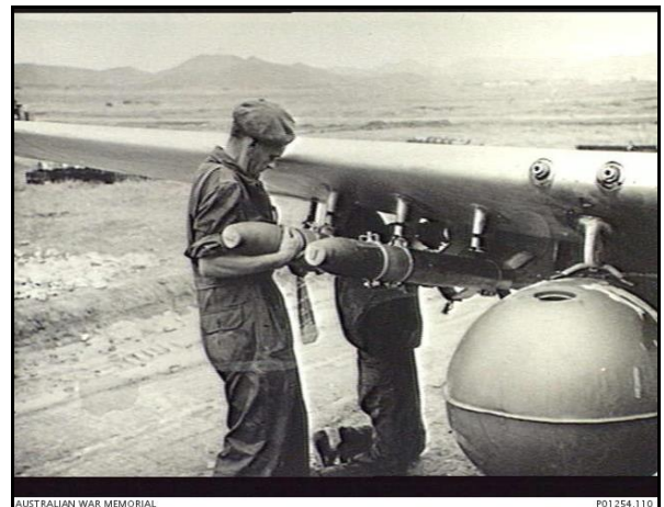
Figure 6 - Armament personnel loading 5" HVAR onto a RAAF Mustang aircraft - Korea (AWM ID number P01254.110)
