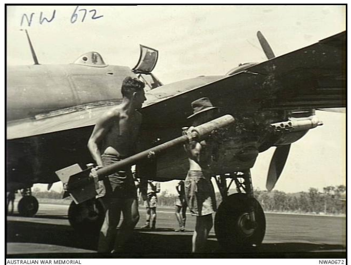
Figure 4 - 60lb concrete head practice rocket being loaded onto a RAAF Beaufighter aircraft at Coomalie Creek, NT in 1944 (AWM ID number NWA0672)
