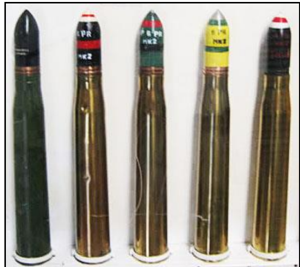
Figure 2 – UK/Aust complete 6 pr munitions showing colours of various types of projectiles (colours & markings may vary)
