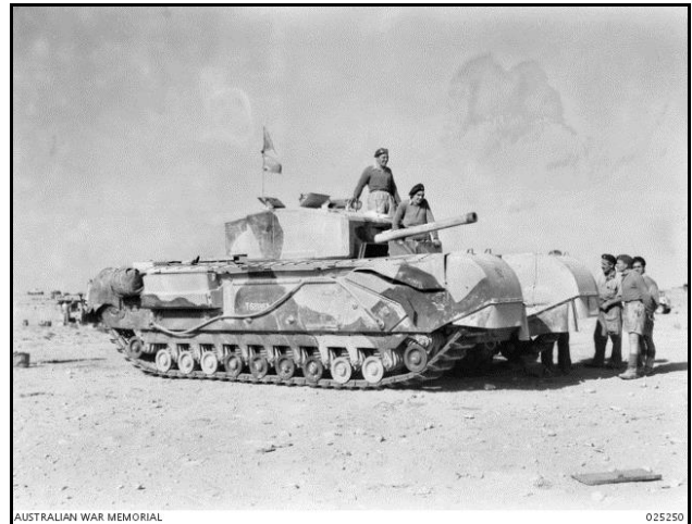
Figure 4 - Churchill IV tanks fitted with a 6 pr gun – Egypt, 1942 (AWM ID number 025250)
