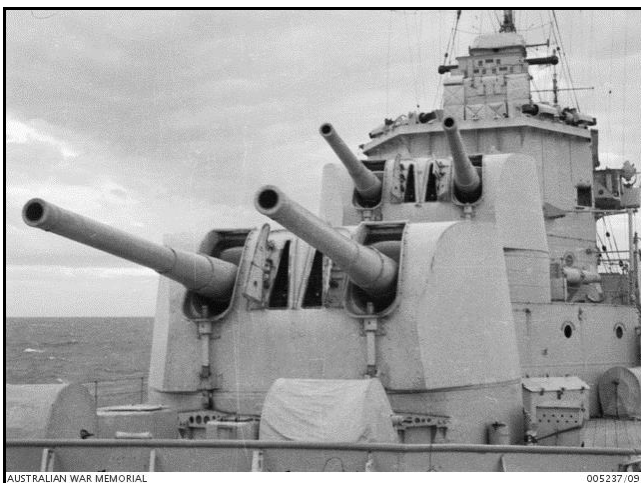
Figure 7 - Twin 6 inch guns on the modified Leander class cruiser HMAS Perth - 1940 (AWM ID number 005237/09)
