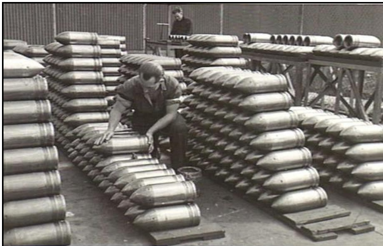
Figure 5 - 6" Armour Piercing projectiles stacked before being filled - 1942 (AWM ID number 013182)
