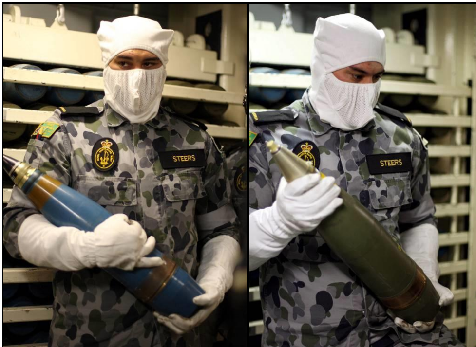
Figure 2 - Australian Navy personnel load 5 inch projectiles during a Naval Gunfire Support exercise - Exercise Talisman Sabre - Shoalwater Bay Training Area, QLD, 2011 (Note differing colours denoting different fillers)
