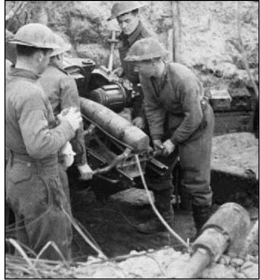
Figure 2 - Loading 5.5 in projectile into the gun breech - Italy, 1944. Image cropped from Imperial War Museums photograph NA 12734)
