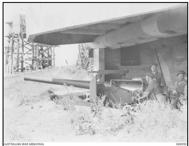
Figure 4 - Australian Coast Gun crew standing by their 4.7 inch QF Mark IV* naval gun at Fort Lytton, Qld - 1943 (AWM ID number 060050)
