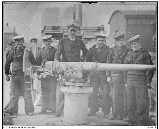
Figure 4 - A Model 1886 3 pr Hotchkiss gun and mount with which motor boats were armed - c 1915 (AWM ID A00911)
