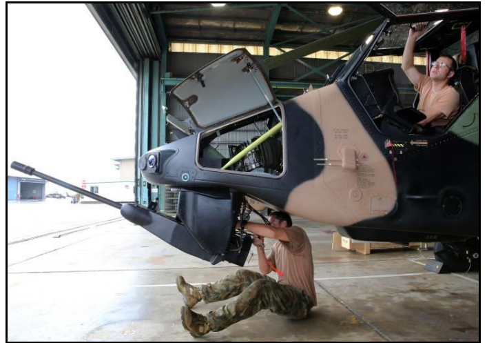
Figure 2 - ADF personnel service a Tiger helicopter's 30 mm cannon
