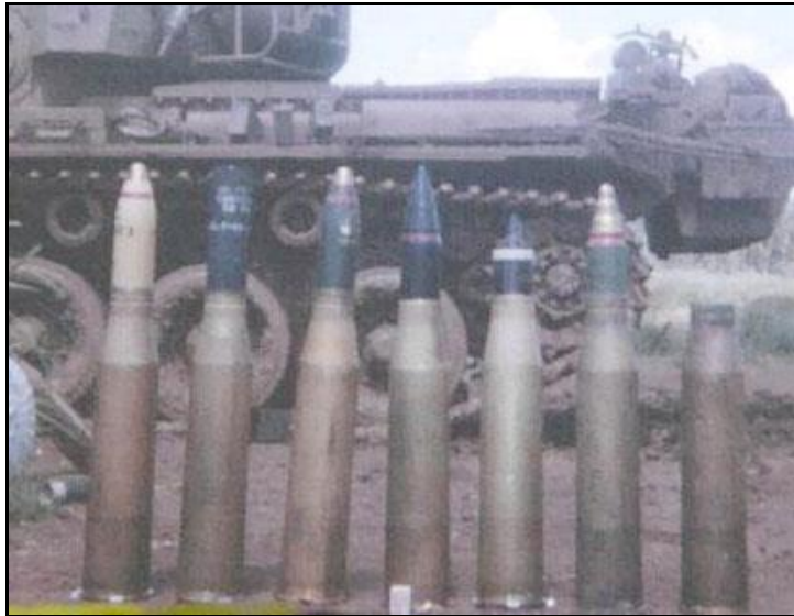
Figure 1 - 20 pr ammunition for Centurian tank (LtoR): HE (yellow), Canister, HE (olive drab), APCBC, APDS, Smk, Blank/empty cartridge
