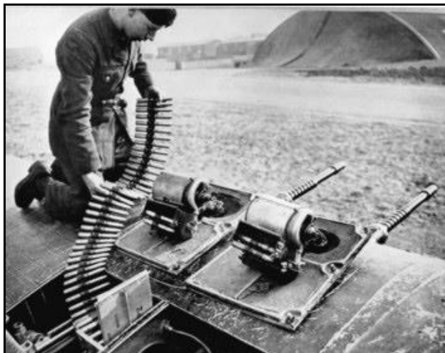
Figure 4 - Belt-fed 20 mm Hispano gun on a Hurricane aircraft
