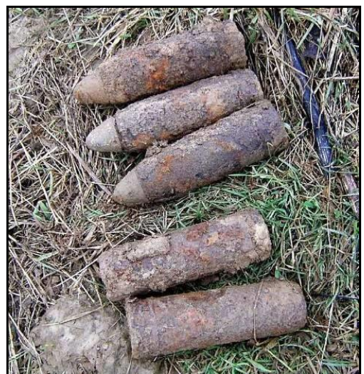
Figure 4 - 18 pr HE/Shrapnel UXO recovered from the field
