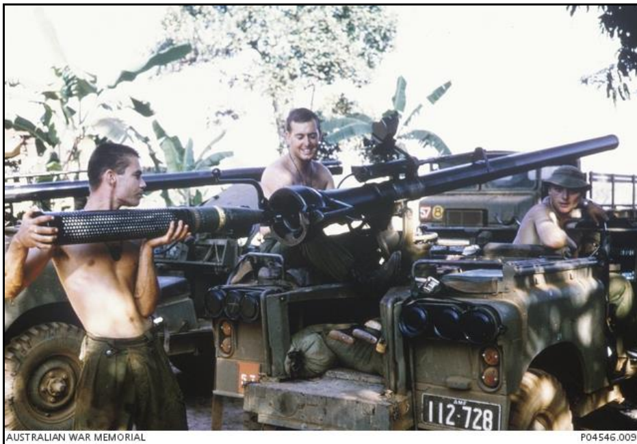
Figure 4 - Australian soldiers from 3 RAR load a HEAT munition into an M40A1 106mm Recoilless rifle mounted on a Land Rover 1/4 ton 4x4 truck (AWM ID P04546.009)
