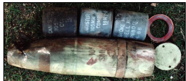
Figure 5 - Expended 105mm Smoke showing expended smoke pots.
