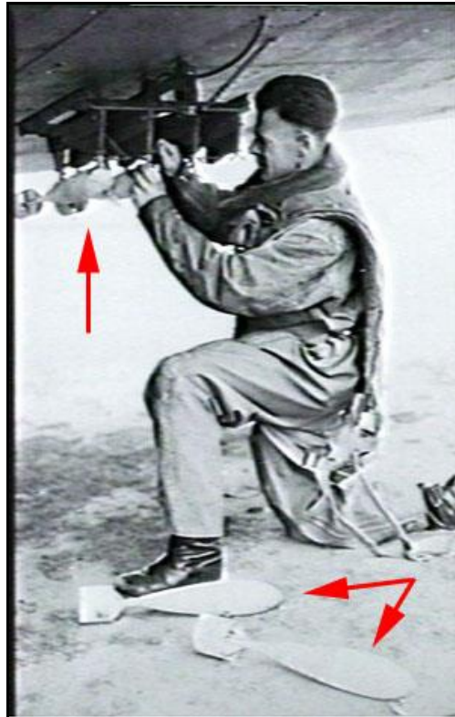
Figure 1 - A RAAF Observer fitting 8 pound Practice Bombs to the bomb rack under a Beaufort Bomber Sale, Vic. 1942. (Photographer Herald Newspaper, AWM ID number 136838)
