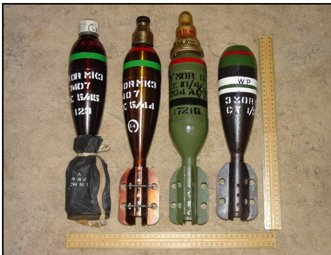
Figure 4 - 3" Mortars - HE, HE (6 vane), Illumination (6 vane), Smoke WP (possibly earlier 3 vane)
